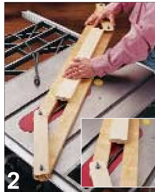
Adjust the cove parallelogram jig so that the inside edges of the jig match the width of the cove profile. Set the jig on the saw table and over the blade. Turn the whole jig left or right until the inside edges of the jig touch the front and back edges of the blade (See inset). In this position, the jig sets the angle you'll need for cutting the cove.
