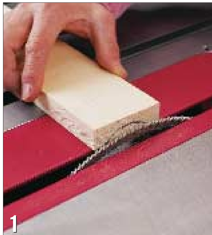
Draw a curved layout line on the end of your workpiece to mark the cove profile. Raise the blade above the saw table so the teeth at the top of the blade match the highest point of the cove profile.
