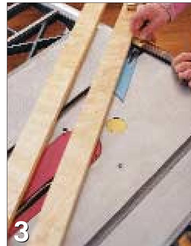
Set a bevel gauge to match the angle the parallelogram jig forms with the front edge of the saw table. Be careful not to bump the parallelogram jig out of alignment as you set the angle on the tool.
