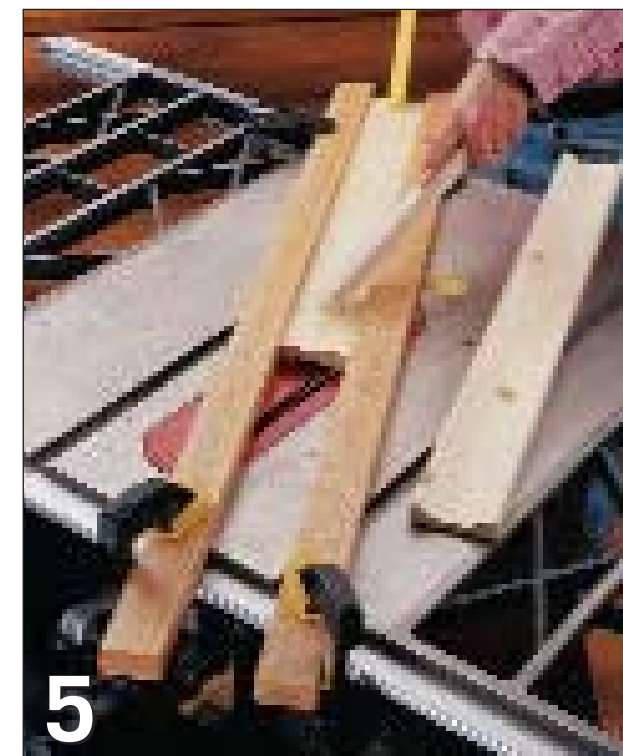
Using the workpiece as a spacer, clamp a second fence to the saw table, parallel to the first fence, to create a track for cutting the workpiece. Then cut the cove in a series of shallow passes, increasing the blade height about 1/16 in. with each pass.
